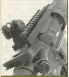
The G.G.&G. Integrated rail system's integral flip-up peep aperture rear sight has two apertures and the sight provides full windage adjustment with a knob on the right side. The flip-up system is controlled by a very positive spring-loaded locking mechanism.
